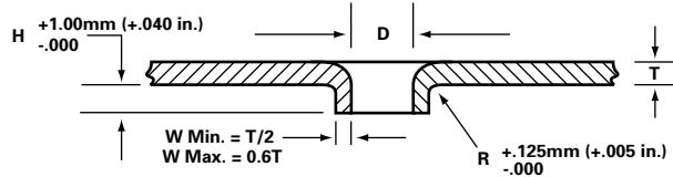
Extruding holes for fasteners in light-gauge steel nearly doubles the length of thread engagement over original material thickness.
